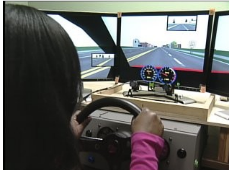
FIGURE 16. Dr. Despina Stavrinos uses driving simulators to study distracted driving. Nine of these presentations and two of these papers resulted from her UTCA Project, #10206, Impact of Distracted Driving on Congestion.
