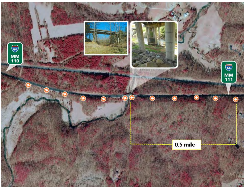
Figure 6. Camera Placement Along Roadside at Site 2. Cameras (represented by circles with arrows indicating the direction the camera faces) are centered above the underpasses and extend 0.5 mile to the east and west.
