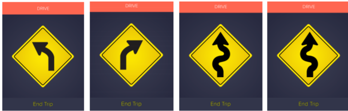
Figure 3.8 Images of advanced curve notifications.
