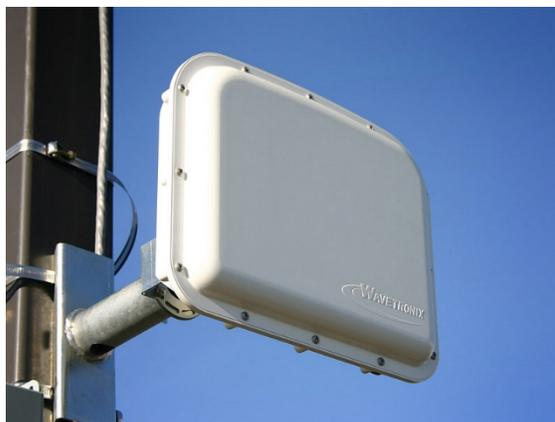
**Figure 3.5** Wavetronix Speed Sensor
