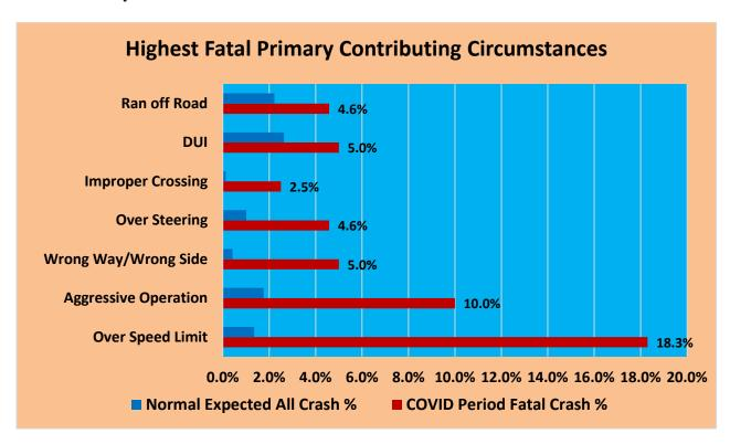
Clearly speed is the primary cause of the increased severity during the COVID period. Surprisingly, crash reports indicate that Aggressive Operation is the second most critical cause. Four of the remaining five are in the 4.6% to 5.0% range, while Improper Crossing (an issue only with pedestrians) is the least frequency, it is still a very important factor in fatality reduction.
