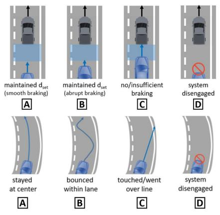
Figure 2. Example codes for the automated longitudinal control features' responses to a slow lead (top) and the lateral control features' responses on curves (bottom) used for classifying participants' qualitative comments.
