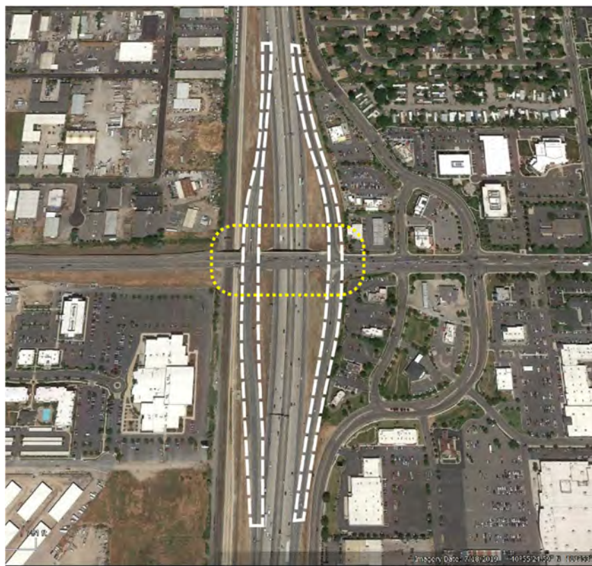
Figure 74. Example of a tight diamond interchange with the ramp boundaries definition
