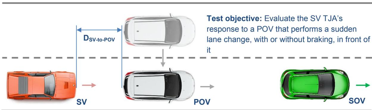
Figure 25. TJA Lead Vehicle Lane Change With Braking (LVLCB) Test Procedure Scenario
