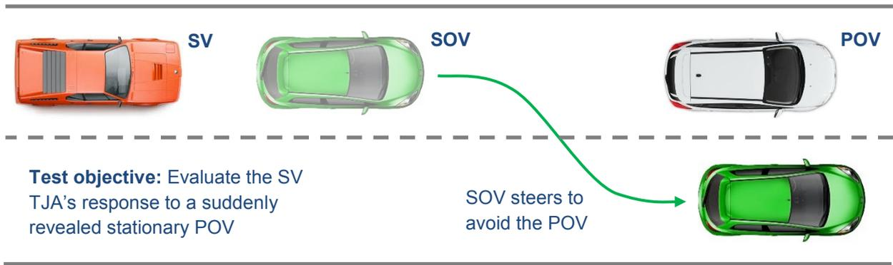
Figure 24. TJA Suddenly Revealed Stopped Vehicle (SRSV) Test Procedure Scenario
