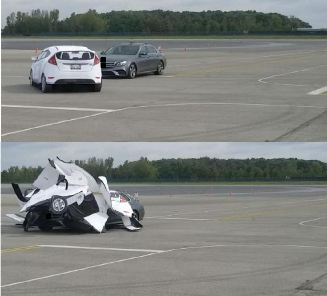
*Figure 23. Execution of ISA LTAP Crash-Imminent Scenario on a Closed-Course Test Track*
