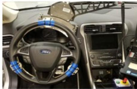
Brake and Accelerator Robot
