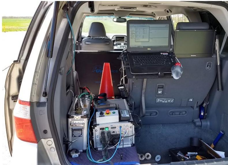
*Figure 10. Support Vehicle With Steering Robot Controller and Laptop*
