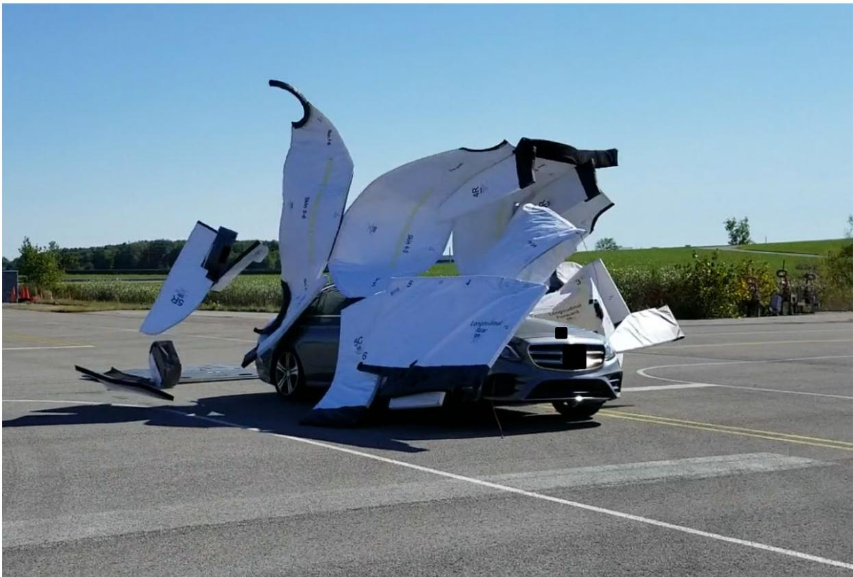
*Figure 20. Execution of ISA SCP Crash-Imminent Scenario on a Closed-Course Test Track*
