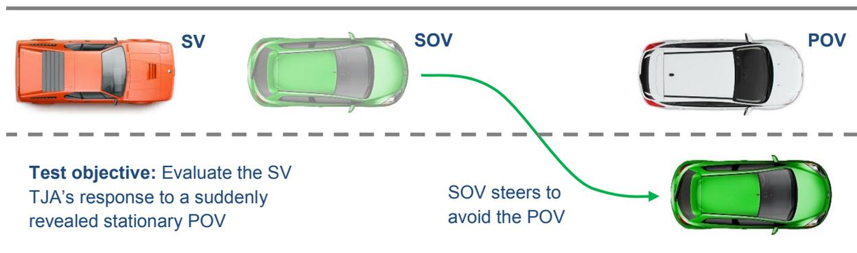
Figure 1. Suddenly Revealed Stopped Vehicle Scenario
