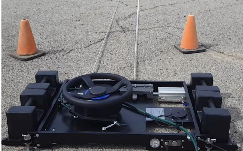
*Figure 9. SPT20 Drive Unit With SR60 Steering Robot*
