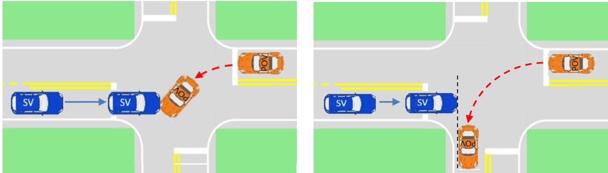
Figure 21. ISA LTAP Test Procedure for Crash-Imminent (top left) and Near-Miss (top right)
