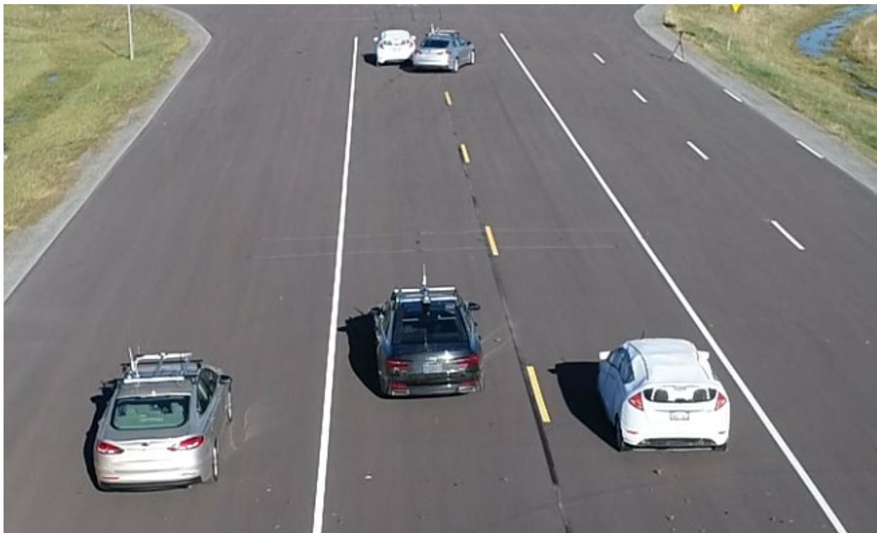
Figure 27. Execution of TJA SRSV Scenario on a Closed-Course Test Track
