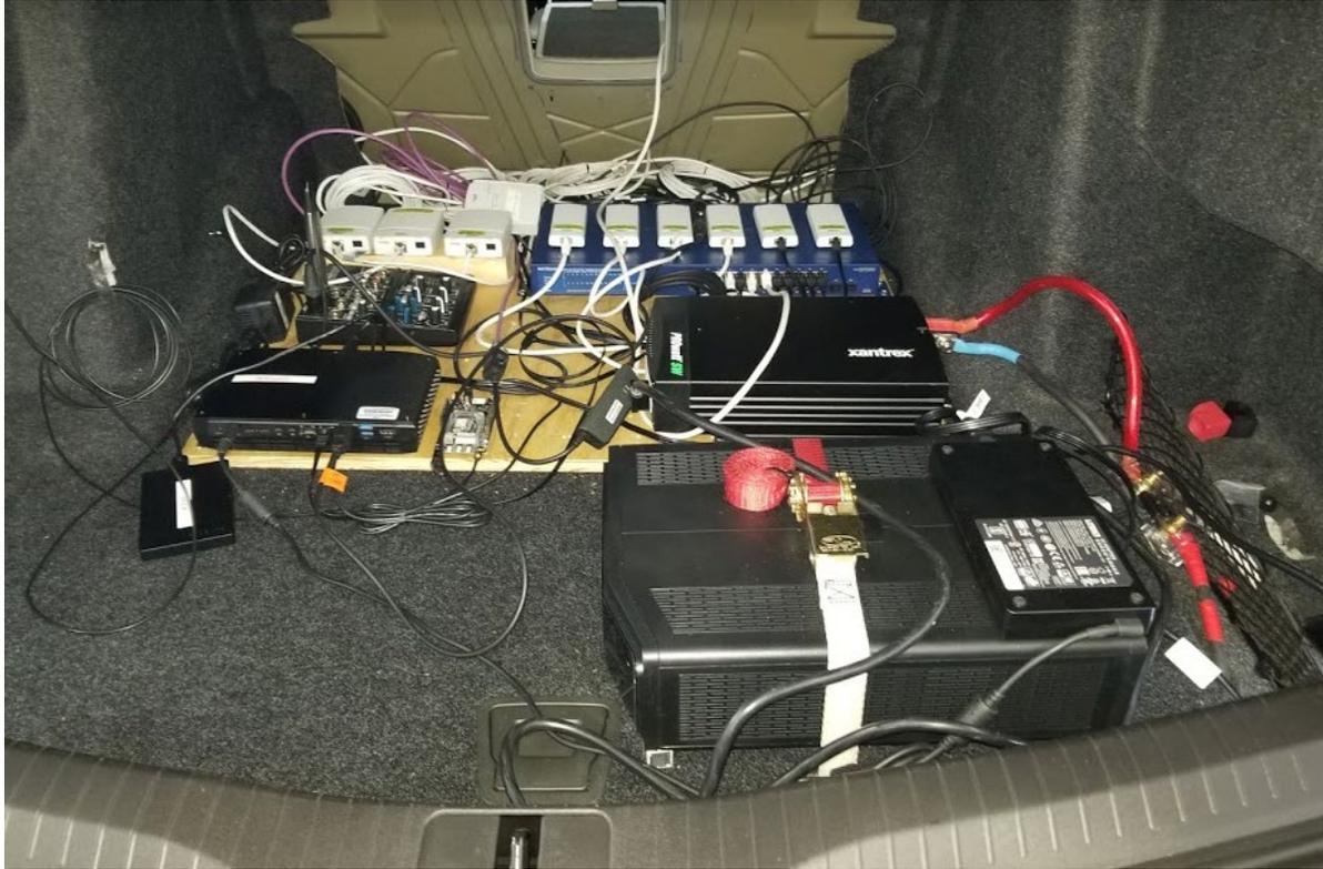
*Figure 15. Robot Operating System Data Acquisition System*
