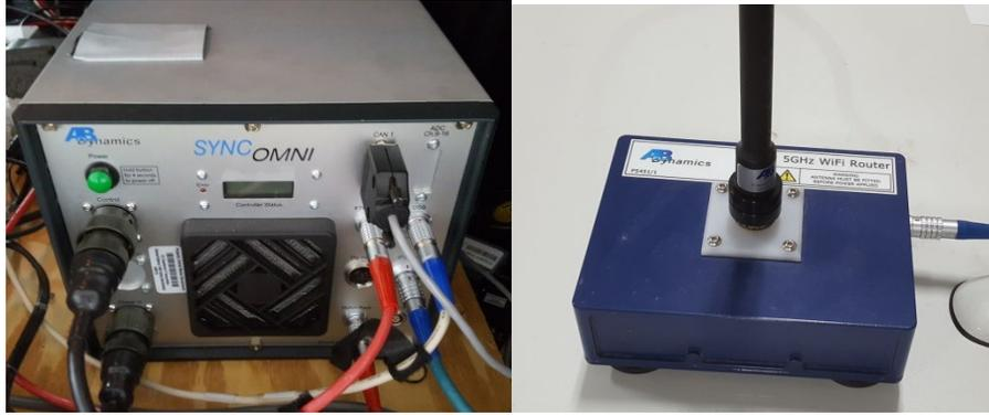
Figure 17. Sync Omni Control Box and TrackFi Antenna
