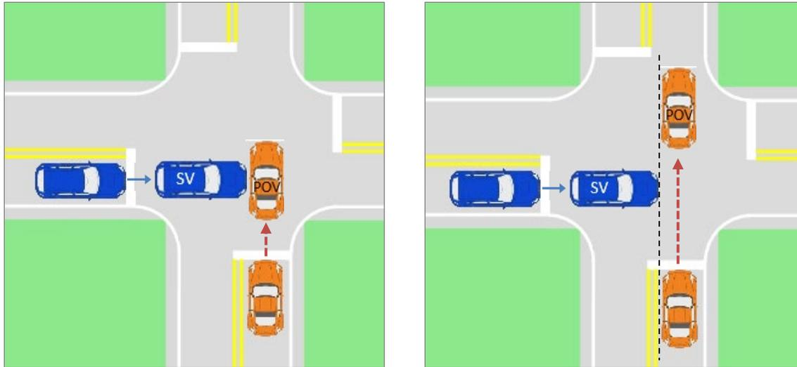
Figure 18. ISA SCP Test Procedure for Crash-Imminent (top left) and Near-Miss (top right)
