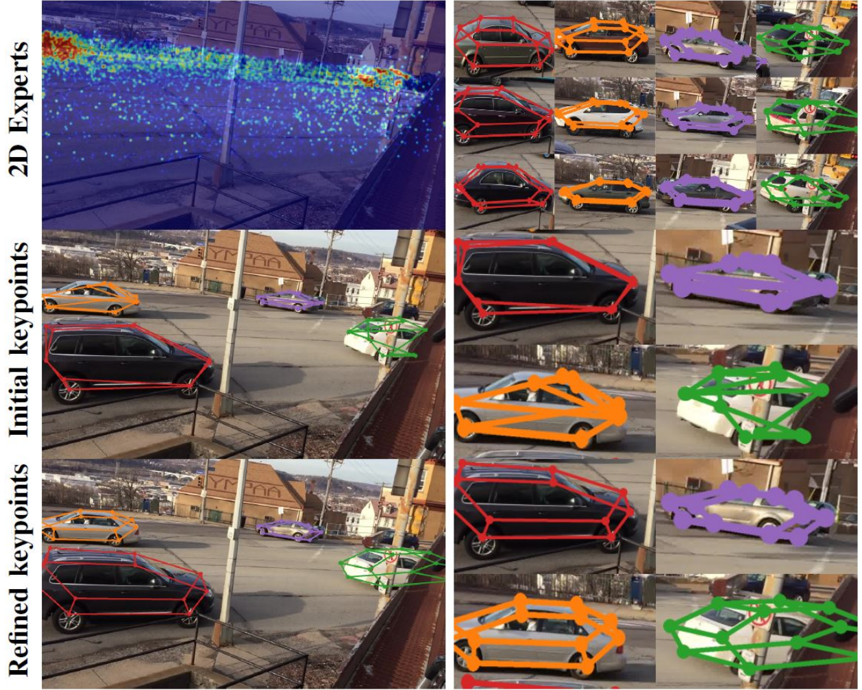
Figure 8: Examples of keypoint refinement via 2D longitudinal self-supervision. First row: Visualization of 2D experts. The heatmaps show frequency of 2D experts being used to refine other instances. 2D experts are used mostly at image border, occluded or far away places. The vehicle patches show the top three nearest neighbors retrieved from expert pool (good keypoints predicted by initial detector); Second row: Initial erroneous keypoints from detector; Third row: Refined keypoints after 2D longitudinal self-supervision.
