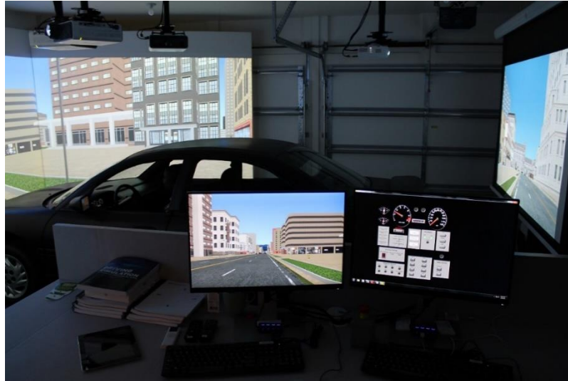
FIGURE 5-3. FULL-CAB DRIVING SIMULATOR AND CONTROL AREA.
